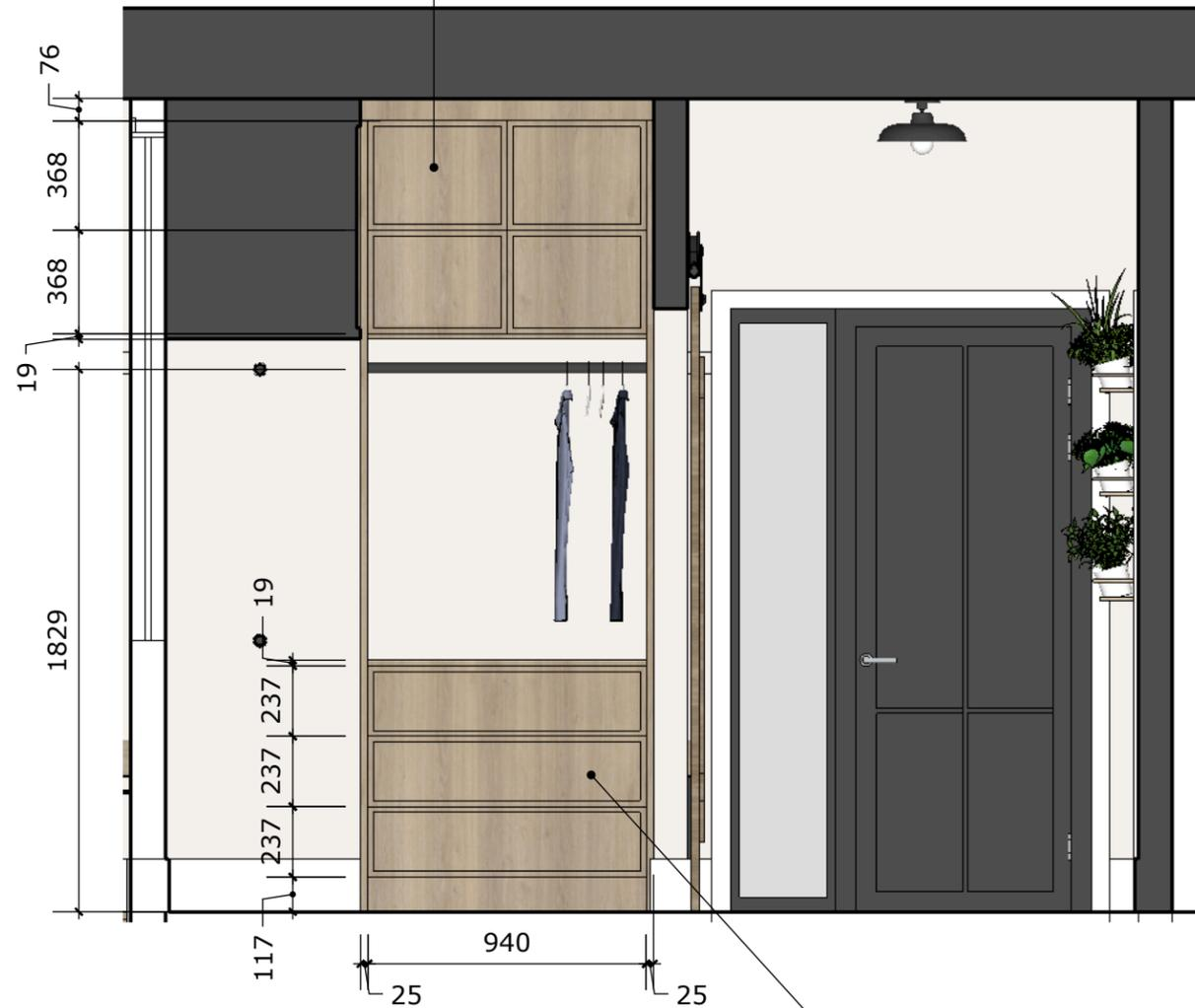
E-2 ÉLÉVATION RANGEMENT SUR MESURE VESTIAIRE
